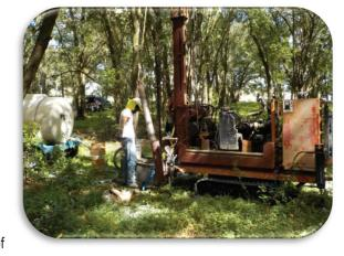
the existing subsurface conditions at the boring locations, to identify constraints or limitations (to the extent possible) that the subsurface conditions may impose on the planned construction and provide general recommendations regarding site suitability, primarily for structures.
