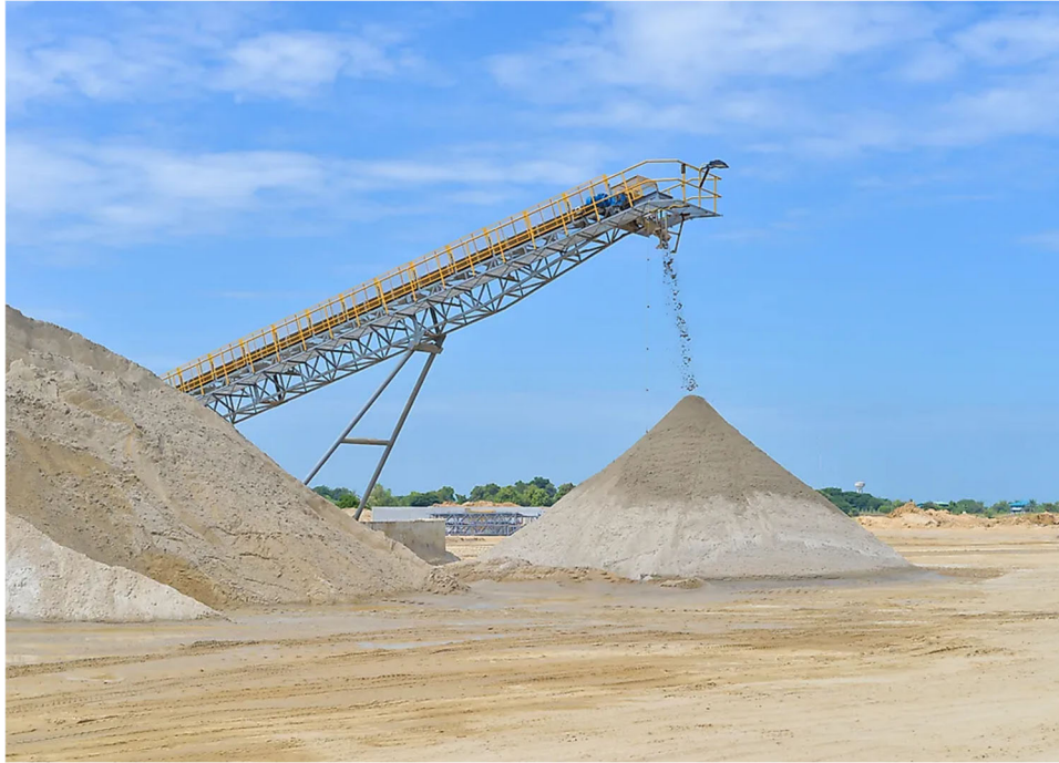
Exhibit 3: Example of conveyor stacking sand for delivery to customers.
