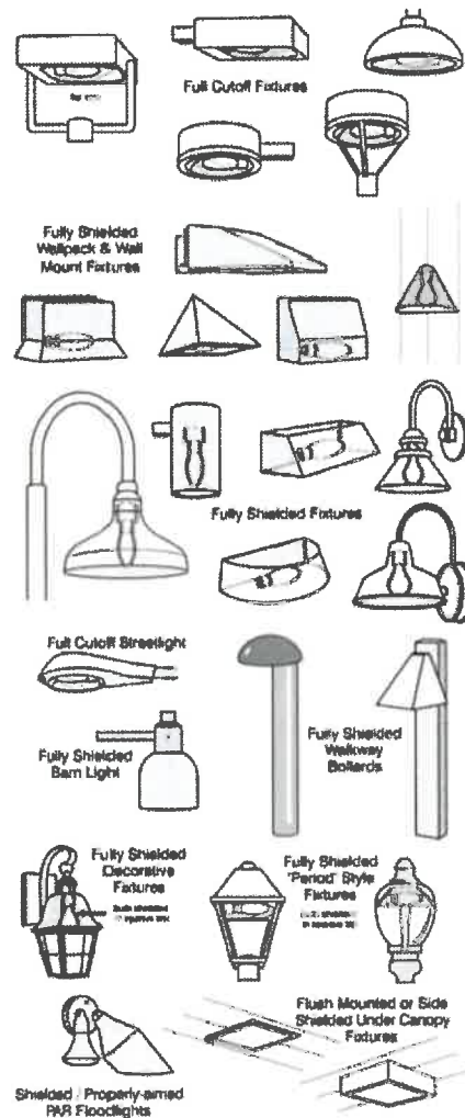
FIGURE "A" EXAMPLES OF FULLY SHIELDED LIGHTS
