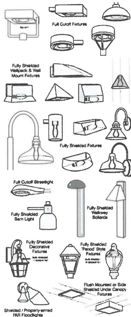
FIGURE "A" EXAMPLES OF FULLY SHIELDED LIGHTS
